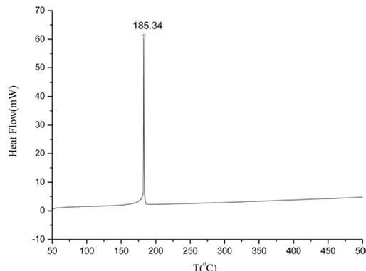
Fig. 1 The DSC curve of compound **2**.
