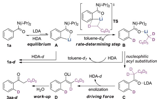
**Scheme 5** A plausible reaction pathway. For clarity, intermediate **A** was showed in its monomer rather than a possible dimer structure (color online).
