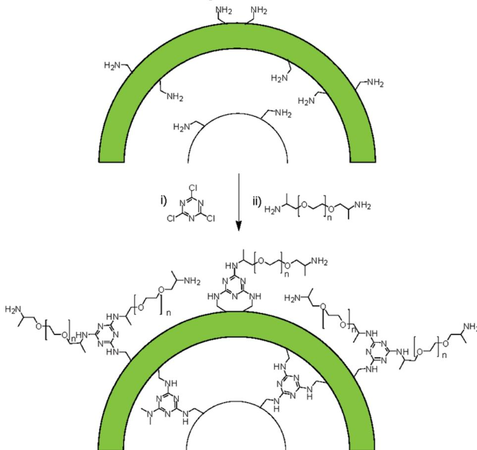
synthesis of novel core–shell (CS) resins readily prepared from commercially available aminomethyl polystyrene (AM-PS, BeadTech<sup>6</sup>) and their characteristics and performances in solid-phase reactions.
