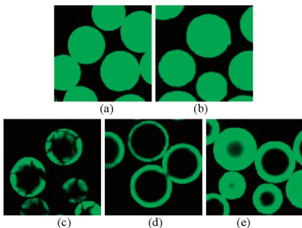
**Figure 1.** Cross-sectioned confocal microscope images of FITC-coupled resins: (a) TentaGel resin (0.3 mmol NH<sub>2</sub>/g); (b) AM-PS resin (0.3 mmol NH<sub>2</sub>/g); (c) CS resin I (0.5–2 equiv of CNC used, 0.03–0.1 mmol NH<sub>2</sub>/g); (d) CS resin II (3–5 equiv of CNC used, 0.2–0.4 mmol NH<sub>2</sub>/g); (e) CS resin III (7–10 equiv of CNC used, 0.5–0.7 mmol NH<sub>2</sub>/g).
