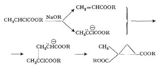
In support of the above mechanism may be cited the fact that application of the Markownikoff-Krestownikoff conditions to a mixture (1:1) of acrylic ester and  $\alpha$ -chloropropionic ester resulted in a several-fold increase in yield of cyclic product. The same acid could also be obtained starting from a mixture of methacrylic ester and chloroacetic ester.
