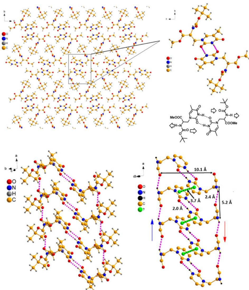
**Figure 3.** Structural studies of single crystal of *N*-Boc-alanyl thymine methyl ester (**3**) by X-ray analysis: (a) Packing diagram (top left); (b) diagram of selected region (top right); (c) Hydrogen bonding pattern (bottom left) and (d) Detail of distance for hydrogen bonding and  $\pi$ - $\pi$  interaction (Bottom right).
