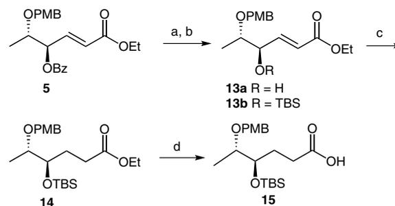
**Scheme 4** Reagents and conditions: (a) K<sub>2</sub>CO<sub>3</sub>, MeOH, r.t., 1 h, 78%; (b) TBSCl, imidazole, CH<sub>2</sub>Cl<sub>2</sub>, 0 °C to r.t., 2 h, 86%; (c) PtO<sub>2</sub>, H<sub>2</sub>, EtOAc, r.t., 3 h, 88%; (d) LiOH, THF–MeOH–H<sub>2</sub>O (3:1:1), r.t., 3 h, 89%.
