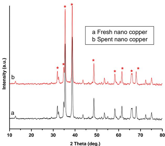
CuO remains CuO under the reaction conditions. This was confirmed by the powder X-ray diffraction analysis exhibited identical peaks for both the fresh and recovered CuO nanoparticles. It is observed that the shape and size of the particles remain unchanged and supports the assumption that the morphology of the catalyst remains the same even after recycling.
