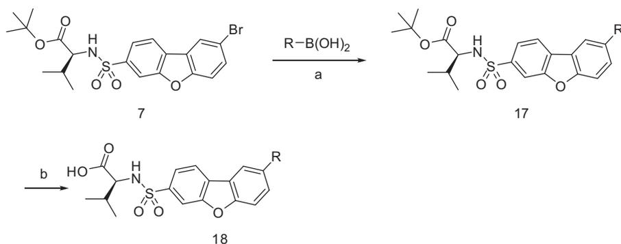
**Scheme 2.** Reagents and conditions: (a) Pd(PPh<sub>3</sub>)<sub>4</sub>, K<sub>2</sub>CO<sub>3</sub>, dioxane, microwave, 120 °C, 15 min, 60–95%. (b) TFA, CH<sub>2</sub>Cl<sub>2</sub>, rt, 6 h, 70–95%.
