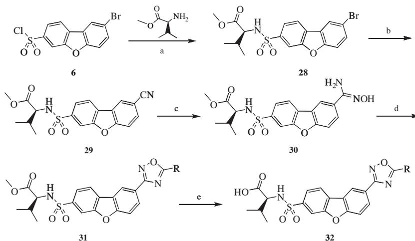
Scheme 3. Reagents and conditions: (a) *i*-Pr<sub>2</sub>NET, CH<sub>2</sub>Cl<sub>2</sub>, rt, 18 h, 92%. (b) CuCN, Pd(PPh<sub>3</sub>)<sub>4</sub>, NMP, microwave, 120 °C, 1 h, 80%. (c) NH<sub>2</sub>OH, TEA, rt, 6 h, 95%. (d) (i) RCOCl, DCM, 0 °C, 2 h, (ii) DMSO, 90 °C, 1 h, 75–88%. (e) LiOH, THF, water, 24 h, 60–95%.
