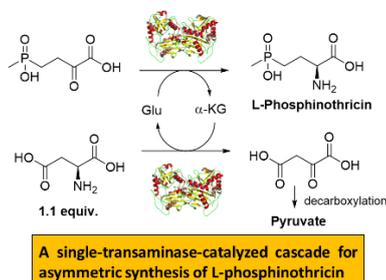
**Asymmetric synthesis of L-phosphinothricin:** A single-transaminase-catalyzed biocatalytic cascade for L-phosphinothricin synthesis was developed by employing a desired biocatalyst ATA-117-Rd11. High conversion, high e.e. of product and low side reaction was achieved by employing only 1.3 equivalent amine donors. In a kilogram-scale experiment, ATA-117-Rd11, about 70 kg L-phosphinothricin (e.e. >99%) was yielded from 80 kg PPO within 24 hours.
