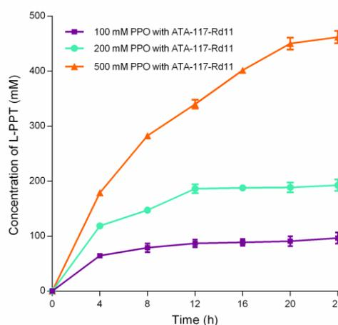
**Figure 2.** Biosynthesis of L-PPT using ATA-117-Rd11 catalyzed cascade toward 100, 200, and 500 mM PPO.
