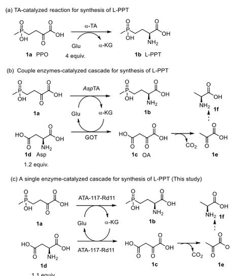
**Figure 1.** The scheme of biosynthesis of L-PPT. (A) a single-TA-catalyzed reaction for synthesis of L-PPT, (B) couple enzymes (TA and GOT)-catalyzed cascade for synthesis of L-PPT, (C) a single enzyme-catalyzed cascade for synthesis of L-PPT
