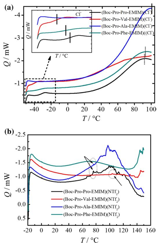
**Fig. 2** DSC curve of synthesized ionic liquid containing chloride and bis(trifluoromethyl)sulfonamide anions
