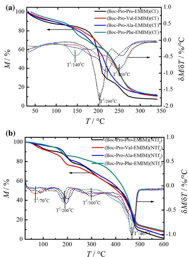
**Fig. 1** TGA (solid line) and DTG (dotted line) of synthesized ionic liquid containing chloride and bis(trifluoromethyl)sulfonamide anions
