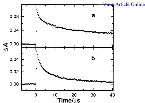
**Fig. 6** Changes in absorbance with time following photolysis of  $3.6 \times 10^{-3} \text{ M CA}$  and  $2.0 \times 10^{-3} \text{ M TA}$  in MeCN solution at (a) 450 and (b) 530 nm.
