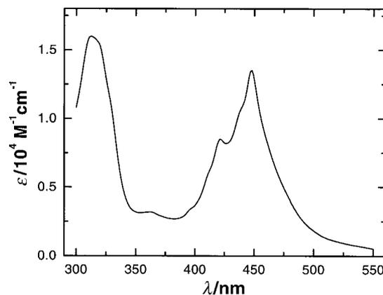
**Fig. 5** Absorption spectrum of  $1 \times 10^{-4}$  M tetrachlorohydroquinone and  $2.4 \times 10^{-4}$  M Me<sub>4</sub>NOH · 5H<sub>2</sub>O in MeCN.
