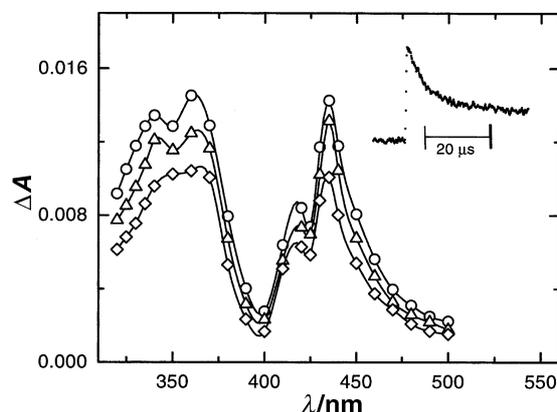
**Fig. 2** Time-resolved absorption spectra obtained by laser photolysis of  $4.0 \times 10^{-3}$  M CA in the presence of  $1.0 \times 10^{-2}$  M TA in  $\text{CH}_2\text{Cl}_2$ , recorded 0.22 (○), 1.9 (△) and 8.0 (◇) μs after the laser pulse ( $\lambda_{\text{exc}} = 355$  nm). Inset: changes in absorbance recorded at 435 nm.
