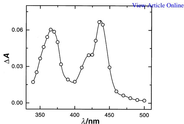
**Fig. 4** Absorption spectrum of CAH<sup>•</sup> obtained by photolysis of CAH<sub>2</sub> (0.025 M) and di-*tert*-butyl peroxide (1 M) in MeCN ( $\lambda_{exc} = 355$  nm).
