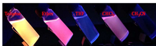
Fig. 1 (a) Normalized absorption spectra of TBMA in different solvents. Solution concentration: 10 \mu M. (b) Photographs of TBMA in different solvents taken under UV illumination at 365 nm.
