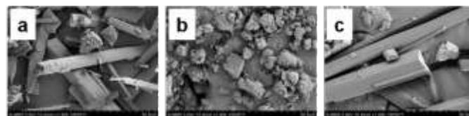
**Fig. 8** SEM images of polymorphs **TSA** (Magnification = 1800). (a) presents the initial sample, (b) presents ground sample and (c) presents sample recrystallized with ethanol.
