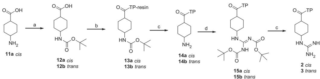
**Scheme 1.** Reagents and conditions: (a) di-*tert*-butyldicarbonate, NaOH, 1,4-dioxane–H<sub>2</sub>O 2:1, 0 °C to room temperature, 3 h. (b) HOBt, HBTU, DIEA, Oic-Pro-*D*-Ala-Phe(*p*-Me)-NH<sub>2</sub> tetrapeptide resin (designated TP-resin), NMP, room temperature, 1.5 h. (c) 95:5 TFA–H<sub>2</sub>O, room temperature, 2 h. (d) *N,N'*-di-Boc-*N'*-triflylguanidine, triethylamine, 1,4-dioxane, room temperature, 24 h.<sup>13</sup>
