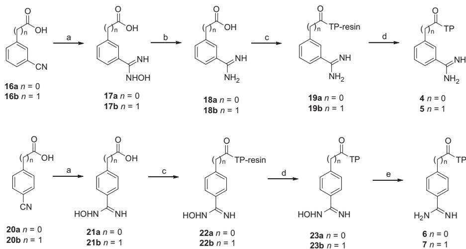
**Scheme 2.** Reagents and conditions: (a) hydroxylamine hydrochloride, KOH, ethanol, reflux, 16–18.5 h.<sup>14</sup> (b) H<sub>2</sub>, 10% Pd/C, H<sub>2</sub>O, 50 °C, 18–20 h. (c) HOBt, HBTU, DIEA, Oic-Pro-*D*-Ala-Phe(*p*-Me)-NH<sub>2</sub> tetrapeptide resin (designated TP-resin), NMP, room temperature, 1–4 h. (d) 95:5 TFA–H<sub>2</sub>O, room temperature, 2 h. (e) acetic anhydride, H<sub>2</sub>, 10% Pd/C, glacial acetic acid, room temperature, 21.5–23.5 h.<sup>14</sup>
