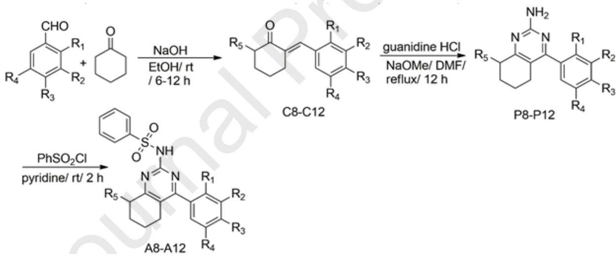
**Scheme 2.** Synthesis of 4-substituted 5,6,7,8-tetrahydroquinazolinyl benzene sulphonamides.
