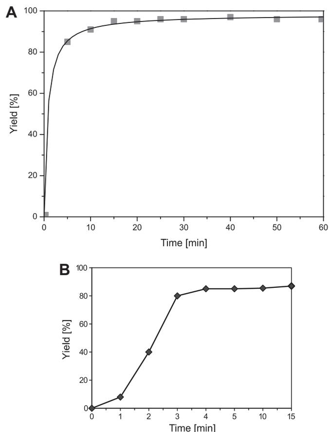
**Fig. 3.** Kinetic profile of Suzuki–Miyaura reaction catalyzed by **3** at 1 mol% (A) and 0.1 mol% (B).
