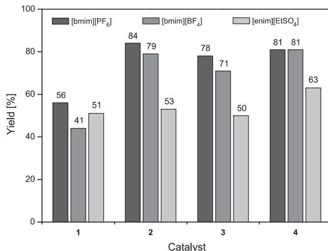
**Fig. 4.** Sonogashira reaction in ionic liquids with catalysts **1–4**.
