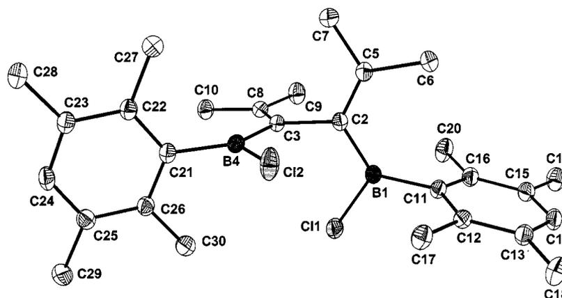
Figure 1. Molecular structure of **4c**; selected bond lengths [Å] (corresponding data for **4e** in square brackets): C3–C8 1.355(3) [1.328(8)], C2–C5 1.360(3) [1.355(8)], C2–C3 1.529(3) [1.520(10), 1.510(11)], C3–B4 1.540(4) [1.574(9)], C2–B1 1.541(4) [1.560(10)], B4–C12 1.799(3) [B–O 1.374(8)] B1–C11 1.802(3) [B–O 1.377(8)], B4–C21 1.582(4) [1.589(9)], B1–C11 1.581(4) [1.590(8)]
