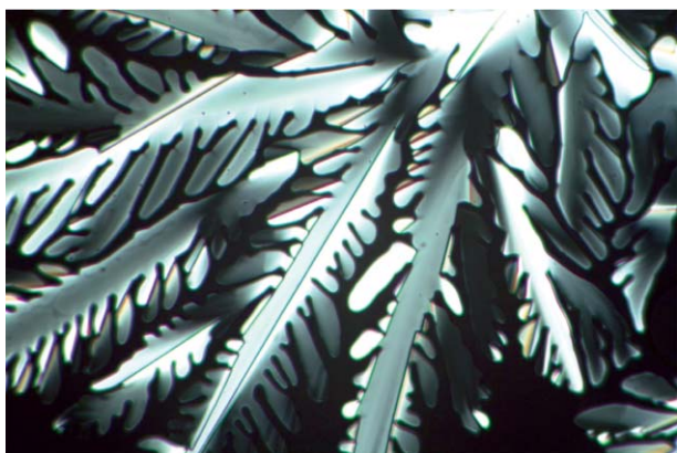
Fig. 2 Optical texture of 3 in the rectangular mesophase.
