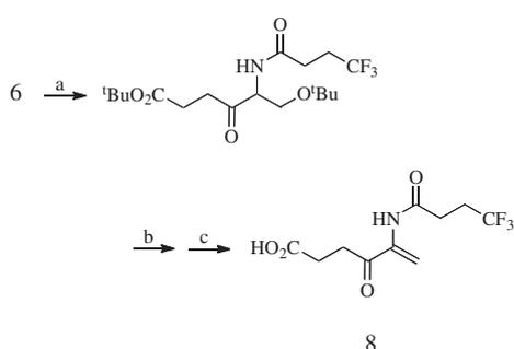
**Scheme 6.** Reagents and conditions: (a) CF<sub>3</sub>CH<sub>2</sub>CH<sub>2</sub>COCl, Et<sub>3</sub>N, CH<sub>2</sub>Cl<sub>2</sub>, rt, overnight, yield 63%; (b) TFA, H<sub>2</sub>O, 0 °C, 3 h, yield 88%; (c) (Boc)<sub>2</sub>O, DMAP, MeCN, rt, overnight then TMG, rt, 24 h, yield 52%.
