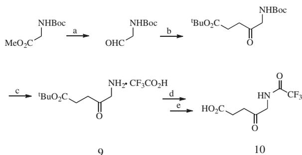
**Scheme 7.** Reagents and conditions: (a) DIBAL-H, toluene, –78 °C, 2 h, yield 82%; (b) 3-ethyl-5-(2-hydroxyethyl)-4-methylthiazolium bromide, *tert*-butyl acrylate, DBU, MS4A, THF, reflux, 12 h, yield 35%; (c) TFA in CH<sub>2</sub>Cl<sub>2</sub>; (d) CF<sub>3</sub>CH<sub>2</sub>CO<sub>2</sub>H, Et<sub>3</sub>N, CH<sub>2</sub>Cl<sub>2</sub>, DMF, (COCl)<sub>2</sub>, yield 75%; (e) TFA, H<sub>2</sub>O, rt, 3 h, yield 55%.
