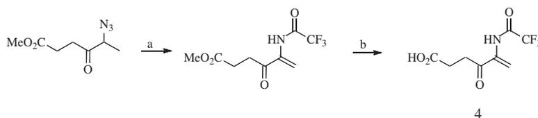
**Scheme 3.** Reagents and conditions: (a)  $\text{NaReO}_4$ ,  $\text{CF}_3\text{SO}_3\text{H}$ ,  $(\text{CF}_3\text{CO})_2\text{O}$ ,  $\text{CCl}_4$ ,  $50^\circ\text{C}$ , 12 h, yield 60%; (b) 1*N* LiOH,  $\text{H}_2\text{O}$ , THF,  $0^\circ\text{C}$ , 1 h, yield 50%.
