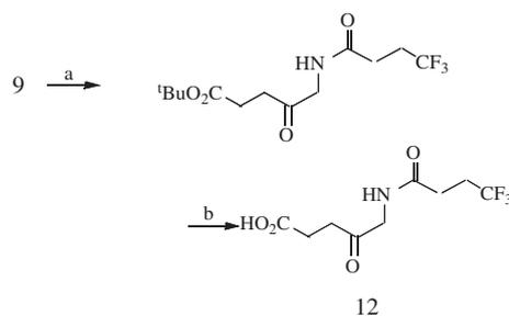
**Scheme 9.** Reagents and conditions: (a) CF<sub>3</sub>CH<sub>2</sub>CH<sub>2</sub>CO<sub>2</sub>H, (COCl)<sub>2</sub>, CH<sub>2</sub>Cl<sub>2</sub>, DMF, Et<sub>3</sub>N, yield 44%; (b) TFA, H<sub>2</sub>O, rt, 3 h, yield 71%.
