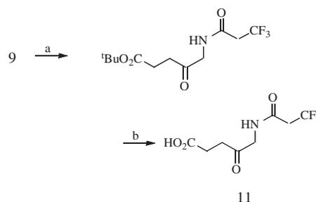
**Scheme 8.** Reagents and conditions: (a) CF<sub>3</sub>CH<sub>2</sub>CH<sub>2</sub>CO<sub>2</sub>H, (COCl)<sub>2</sub>, CH<sub>2</sub>Cl<sub>2</sub>, DMF, Et<sub>3</sub>N, yield 74%; (b) TFA, H<sub>2</sub>O, rt, 3 h, yield 88%.
