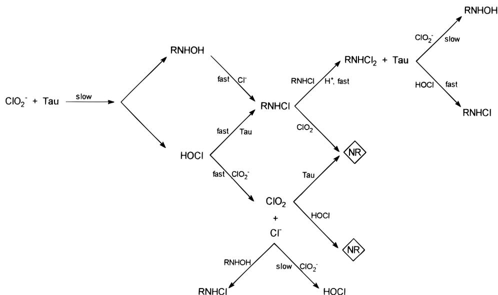
**Figure 7.** Schematic diagram showing the various reactions involved in the chlorite–taurine reaction.  $\text{ClO}_2(\text{aq})$  acts as a Cl(IV) sink as it undergoes no further reaction with any other species in solution except  $\text{Cl}^-$ . Tau represents taurine,  $\text{RNHCl}$  is taurine monochloramine,  $\text{RNHCl}_2$  is taurine dichloramine, and,  $\text{RNHOH}$  is the hydroxylamine formed from taurine while NR stands for no reaction.
