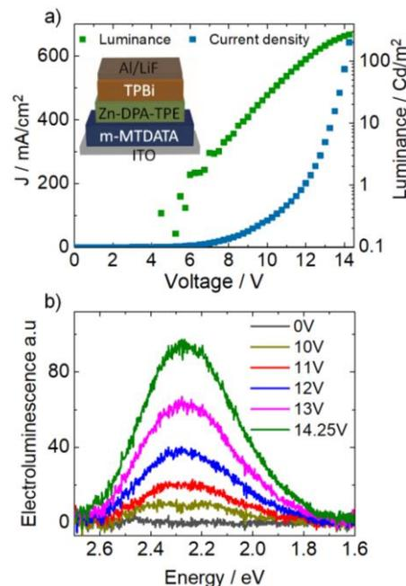
**Figure 3.** a) Current density and luminance of **1**, with different applied voltages, inset: LED device structure of **1**; b) Electroluminescence spectra of **1** obtained at different applied voltages, using a device configuration shown above; (a.u. = arbitrary unit).
