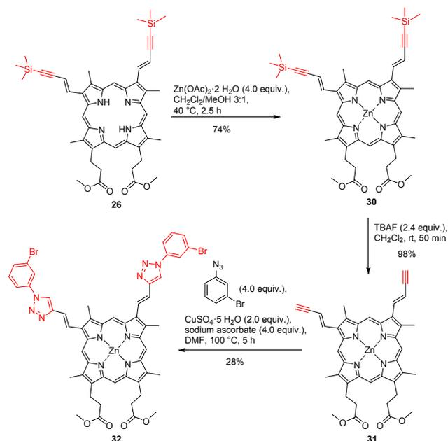
**Scheme 9.** Functionalization of a protoporphyrin IX derivative (**31**) by azide-alkyne 1,3-dipolar cycloaddition to give **32**.
