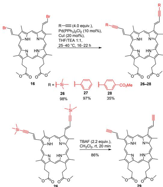
**Scheme 8.** Sonogashira coupling reactions between **16** and different ethynyl substrates to give **26–28** and deprotection of **26** with TBAF to give **29**.
