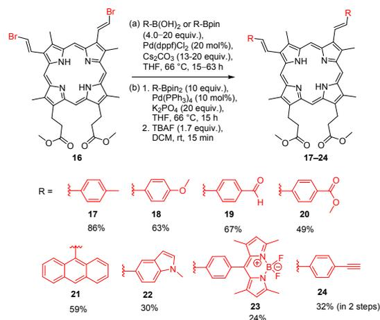
**Scheme 5.** Suzuki-Miyaura coupling reactions of **16** with different boronic acids and boronic acid pinacol esters to yield **17–24**.
