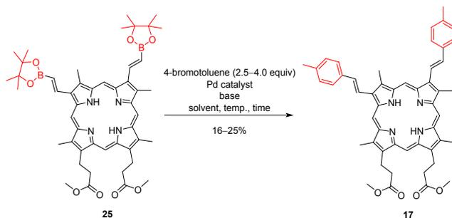
**Scheme 7.** Suzuki-Miyaura cross-coupling reactions of **25** with 4-bromotoluene to give **17**.
