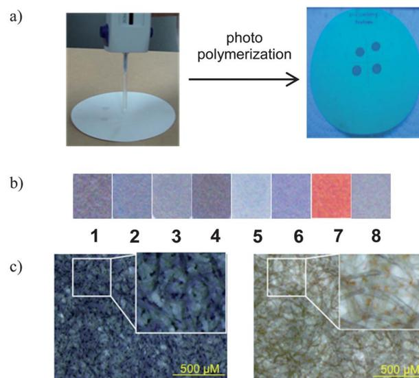
Fig. 2 (a) Preparation of paper-based PDA sensor and (b) scanned images of sensor array constructed from 1–8 exposed with UV light (1 min, 500  $\mu\text{W cm}^{-2}$ ). (c) Microscopic images of a paper based PDA sensor from 8 before (left) and after exposure to THF vapor (right).
