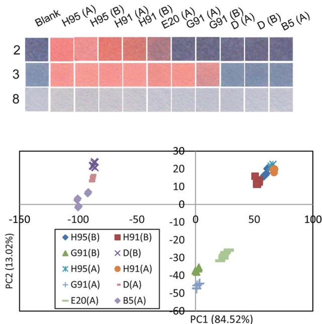
**Fig. 6** (Top) Scanned images of the paper-based PDA sensor array prepared from **2**, **3** and **8** before (blank) and after exposure to 10 automotive fuel vapors. (Bottom) PCA score plot of RGB color changes obtained from the paper-based PDA sensor array derived from **2** and **3** upon exposure to automotive fuels (2 PDAs  $\times$  3 replicates  $\times$  10 automotive fuels  $\times$  3 measurements of each RGB).
