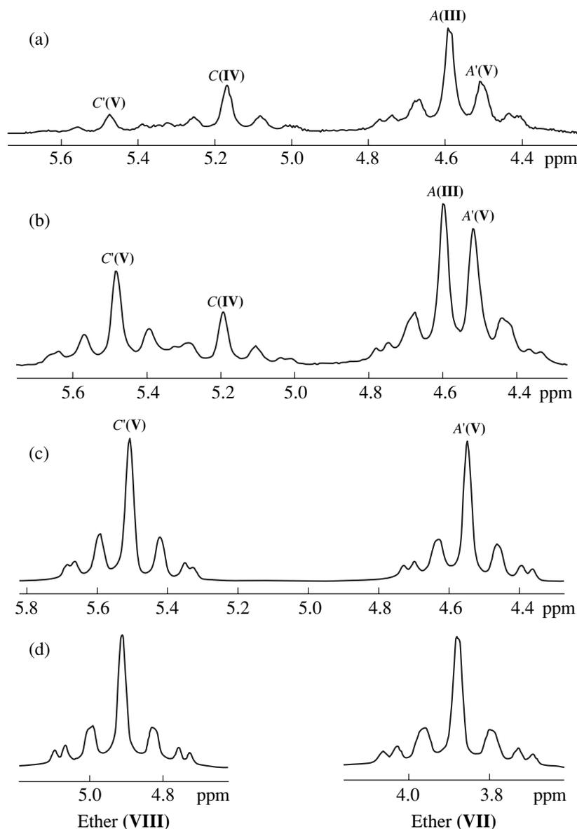
**Fig. 2.** Parts of  $^{19}\text{F}$  NMR spectra of the reaction mixtures presented in Scheme 1 that correspond to  $\beta, \beta'$ -fluorine atoms of pyridyl rings A, C, A', and C' of (III), (IV), and (V). The spectra were registered after (a) 0.75, (b) 3, and (c, final) 16 h; (d), the parts of  $^{19}\text{F}$  NMR spectra of the reaction mixtures corresponding to  $\beta, \beta'$ -fluorine atoms of pyridyl rings of ethers (VII) and (VIII)
