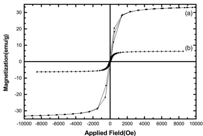
**FIGURE 5** VSM patterns of (a)  $\text{Fe}_{3-x}\text{Ti}_x\text{O}_4$  and (b)  $\text{Fe}_{3-x}\text{Ti}_x\text{O}_4$ @SPDETATSA MNPs
