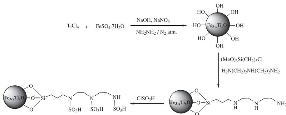
**SCHEME 1** Preparation of Fe<sub>3–x</sub>Ti<sub>x</sub>O<sub>4</sub>-supported *N*-(3-silyl propyl) diethylene triamine *N,N,N'*-tri-sulfonic acid nanoparticles (Fe<sub>3–x</sub>Ti<sub>x</sub>O<sub>4</sub>@SPDETATSA)
