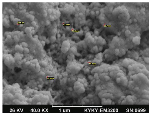
**FIGURE 3** Scanning electron microscopy (SEM) image of  $\text{Fe}_{3-x}\text{Ti}_x\text{O}_4$ @SPDETATSA MNPs
