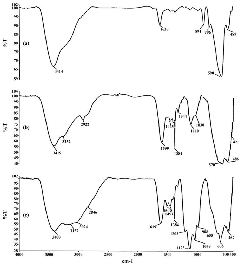
**FIGURE 1** FT-IR spectra of: (a)  $\text{Fe}_{3-x}\text{Ti}_x\text{O}_4$  MNPs, (b)  $\text{Fe}_{3-x}\text{Ti}_x\text{O}_4$ @SPDETA MNPs and (c)  $\text{Fe}_{3-x}\text{Ti}_x\text{O}_4$ @SPDETATSA MNPs
