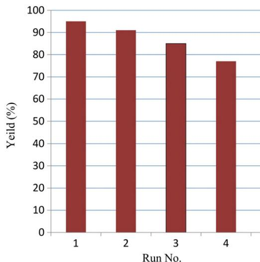
**FIGURE 7** Recyclability of the catalyst ( $\text{Fe}_{3-x}\text{Ti}_x\text{O}_4$ @SPDETATSA) in the synthesis of **5a** under the optimized condition
