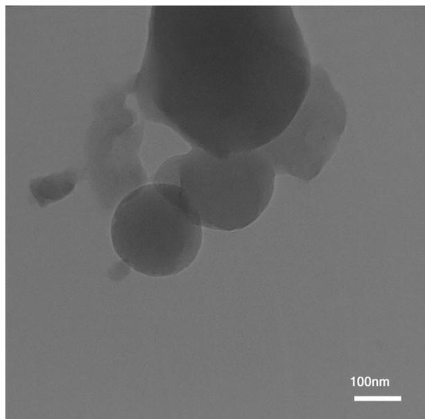
**FIGURE 4** Transmission electron microscopy (TEM) image of  $\text{Fe}_{3-x}\text{Ti}_x\text{O}_4$ @SPDETATSA MNPs
