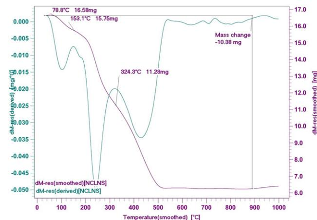
**FIGURE 6** TGA and DTA curves of the  $\text{Fe}_{3-x}\text{Ti}_x\text{O}_4$ @SPDETATSA nanocatalyst
