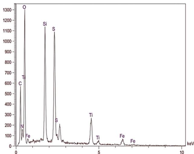
**FIGURE 2** EDX pattern of the  $\text{Fe}_{3-x}\text{Ti}_x\text{O}_4$ @SPDETATSA MNPs
