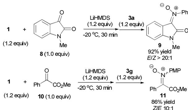
**Scheme 4** Phosphite-initiated nitrone formation from *N*-methyl isatin **8** and methyl benzoylformate **10**.
