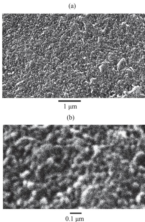
**Fig. 1.** Electron micrographs of the TiO<sub>2</sub>-SiO<sub>2</sub> surface.
