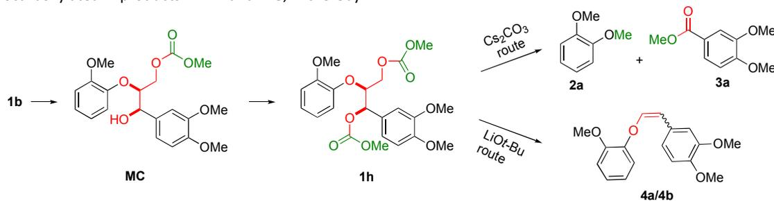
**Scheme 4** Reaction of the  $\beta$ -O-4 model linkage under BCD conditions showing the reaction sequence and the point of divergence in reactivity for  $\text{Cs}_2\text{CO}_3$  and  $\text{LiOt-Bu}$ .
