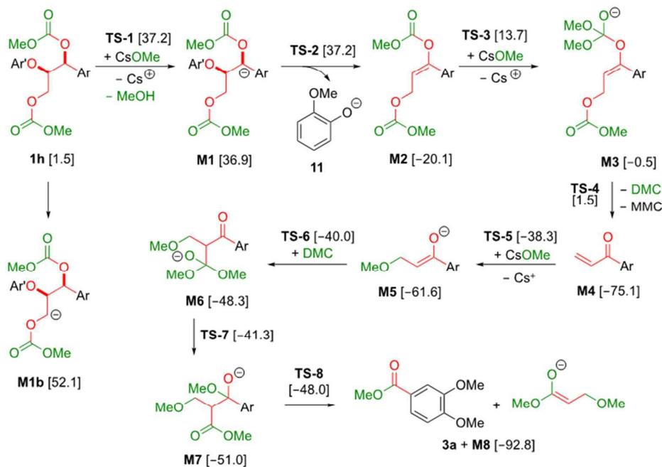
**Scheme 5** Reaction pathway from dicarboxylated Dilignol **1h** to 3,4-dimethoxy benzoate (**3a**); Ar: 3,4-dimethoxyphenyl; Ar': 2-methoxyphenyl; MMC: monomethoxy carbonate; [Gibbs Energies Relative to **1b** in kcal mol<sup>-1</sup>]
