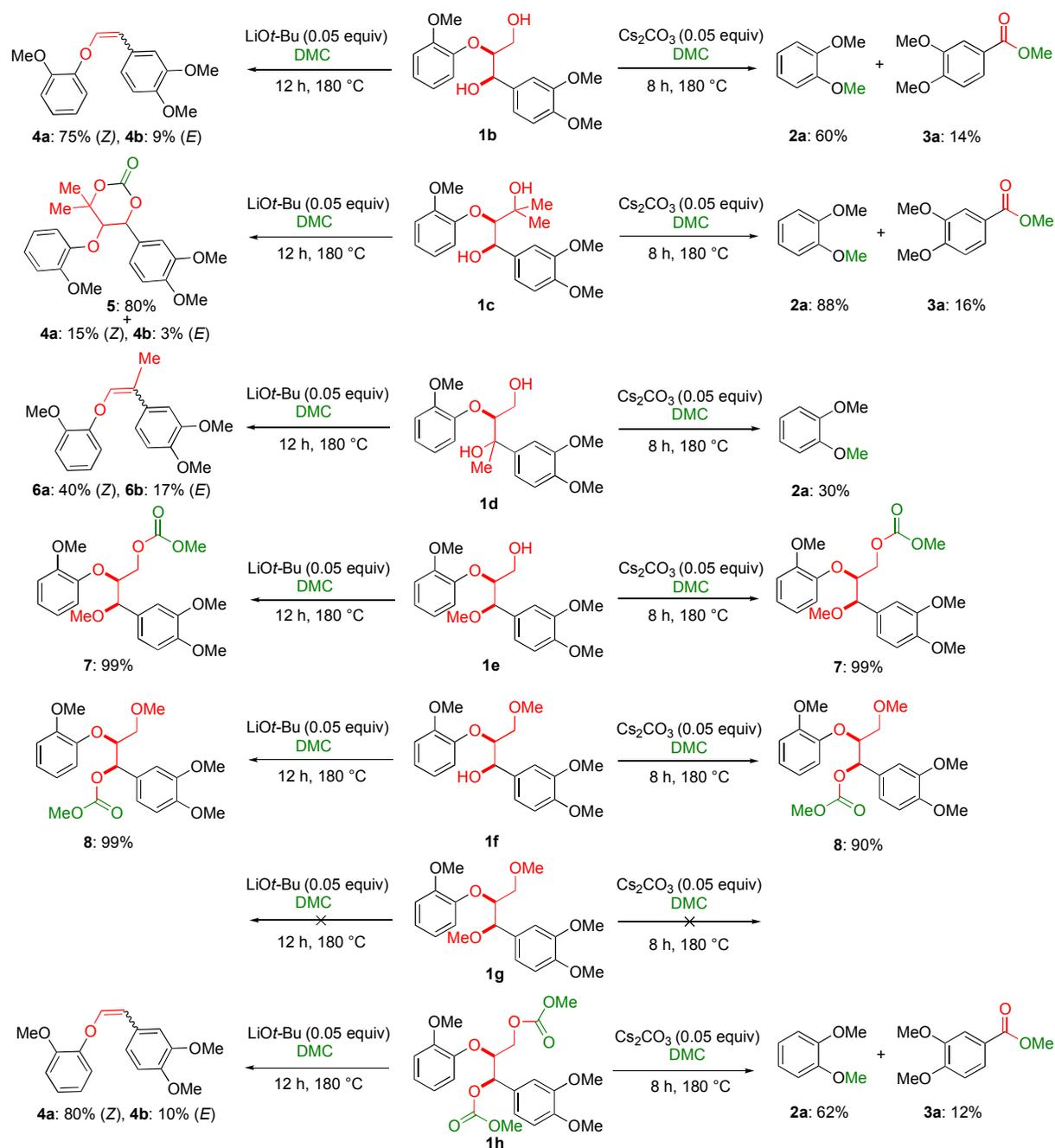
**Scheme 3** Base-catalysed degradation in lignin  $\beta$ -O-4 model compounds.
