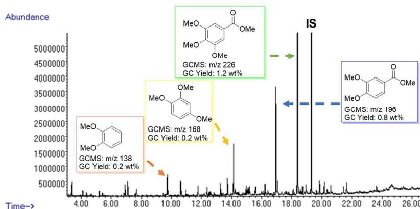
**Fig. 4** GC-FID trace of the product mixture obtained from the depolymerisation of milled beechwood chips (100 mg) using Cs<sub>2</sub>CO<sub>3</sub> (10 wt %) in DMC (5 mL) at 180 °C for 8 h. Identification of the major peaks is based on the GC-MS data (full peak overview in Table S6). Quantification is based on the standardization of individual products, using *n*-octadecane as an internal standard.
