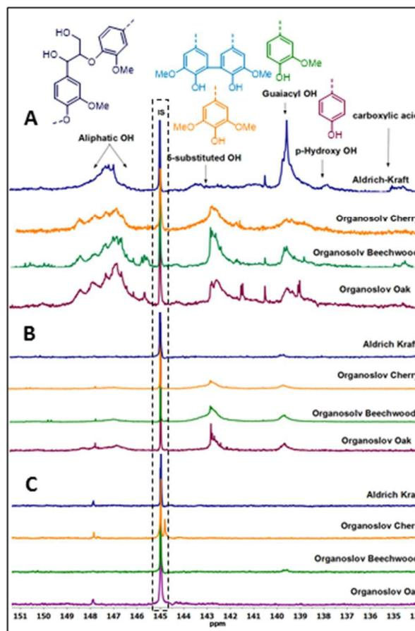
**Fig. 2** Quantitative  $^{31}\text{P}$  NMR spectra of lignins; **A** before the reaction; **B** after the reaction with LiOt-Bu; **C** after the reaction with  $\text{Cs}_2\text{CO}_3$ .
