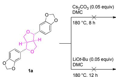
**Scheme 2** Reactivity of  $\beta$ - $\beta$  model compound **1a** in the BCD reactions.
