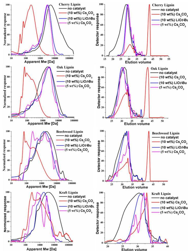
**Fig. 3** GPC measurements for the cherry, oak, beechwood and Kraft lignin samples: before reaction (no catalyst); after reaction with  $\text{Cs}_2\text{CO}_3$  (10 wt%, 0.030 mmol), 8 h, 180 °C; after reaction with LiOt-Bu (10 wt%, 0.125 mmol), 12 h, 180 °C; after reaction with  $\text{Cs}_2\text{CO}_3$  (5 wt%, 0.015 mmol), 8 h, 180 °C. **Left:** mass distribution with respect to polystyrene standards calibration; **Right:** elugram.
