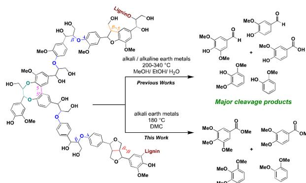
Scheme 1 Base-catalysed cleavage of lignin in DMC.
