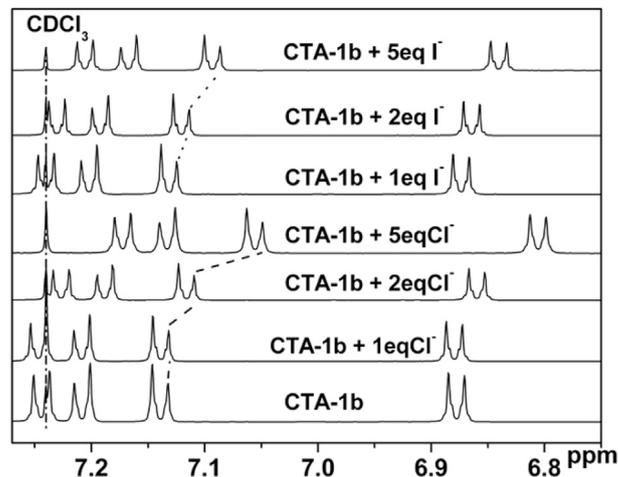
**Fig. 3.**  $^1H$  NMR spectra (aromatic region) of **CTA-1b** upon titration with TBACl and TBAI ( $CDCl_3$ , 298 K).
