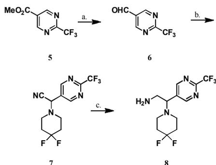
**Scheme 2:** Synthesis of compounds **1a-1i**: a. DIBAL, -78 °C, DCM; b. 4,4-difluoropiperidine hydrochloride, Me<sub>3</sub>SiCN, acetic acid, 45% over 2 steps; c. Raney Nickel, 7N NH<sub>3</sub> in methanol, H<sub>2</sub> (45 psi), MeOH, 98%.
