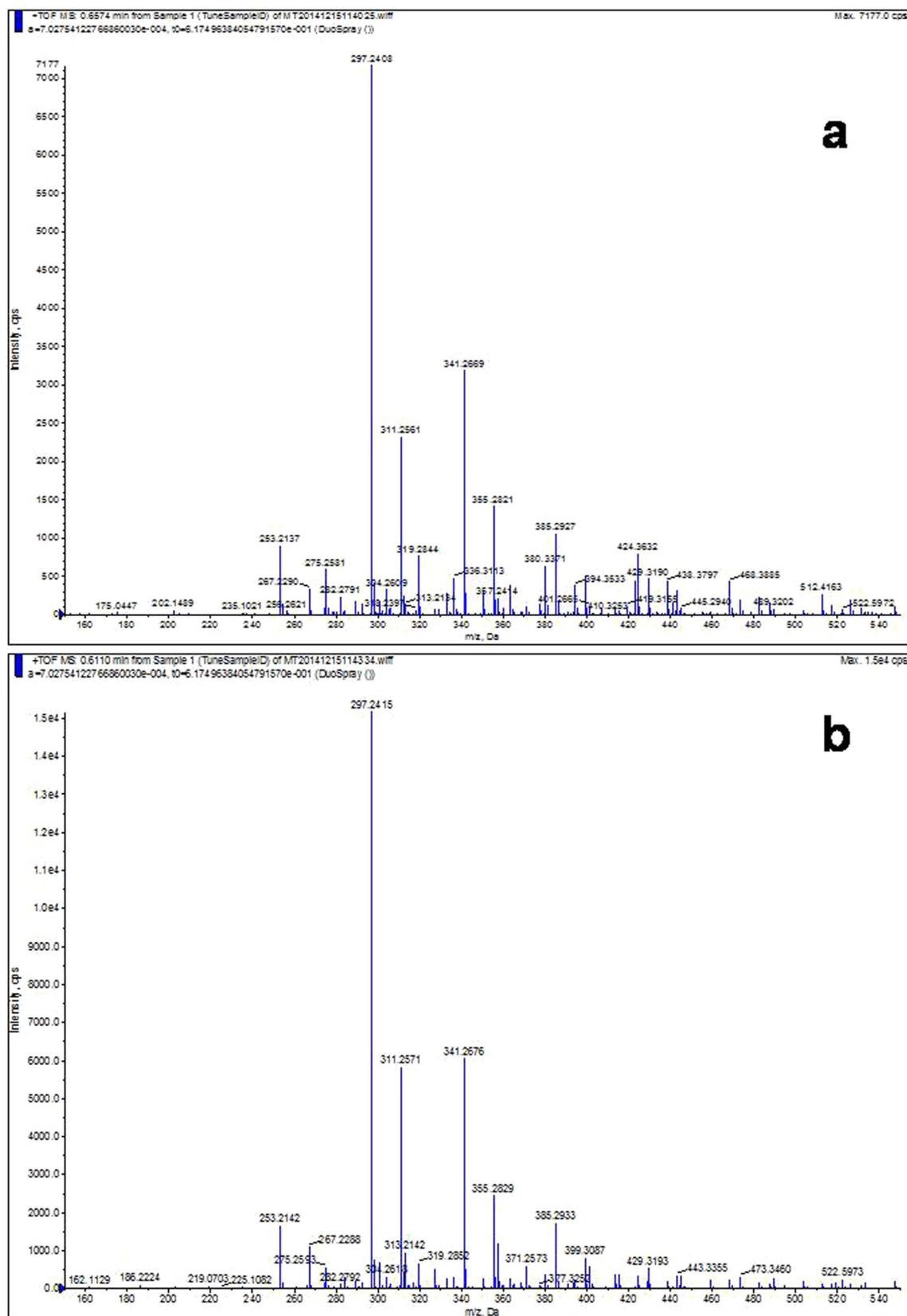
**Fig. 4.** Representative mass spectra of degradation product T8 (a) and T10 (b) after individual injection in mass spectrometer operating by positive electrospray ionization. Injection volume of 10  $\mu$ L and temperature of 300  $^{\circ}$ C.
