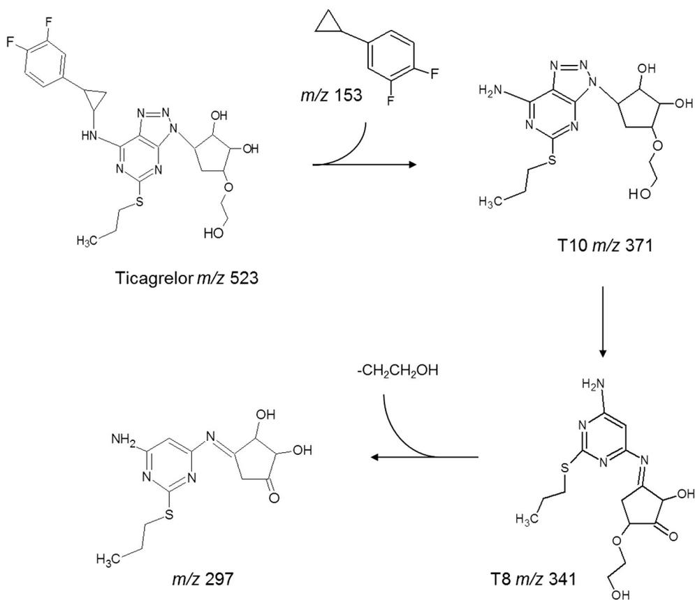
Fig. 5. Proposed photolytic degradation routes with the chemical structures of the T10 and T8 degradation products.
