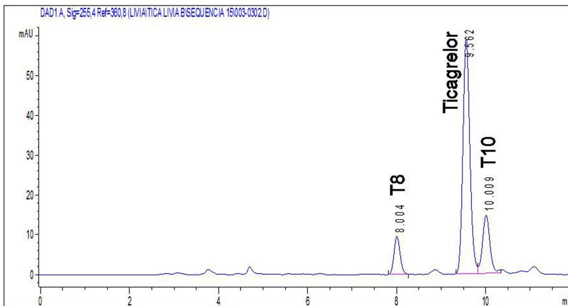
**Fig. 3.** Representative chromatogram of ticagrelor and two major degradation products after UVC light exposure for 2 h. Chromatographic conditions: C18 Phenomenex Luna column (250 × 4.6 mm, 5.0  $\mu\text{m}$ ) at 25 °C, with a mobile phase consisting of acetonitrile: water (57:43 v/v), at a flow rate of 0.7  $\text{mL} \cdot \text{min}^{-1}$  and injection volume of 20  $\mu\text{L}$ . The detection was made at a wavelength of 255 nm by using PDA detector.
