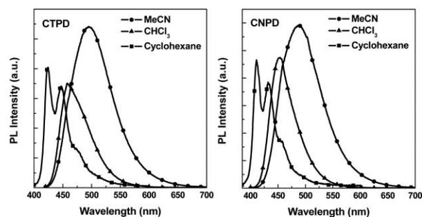
Fig. 6 Photoluminescence spectra of CTPD and CNPD.
