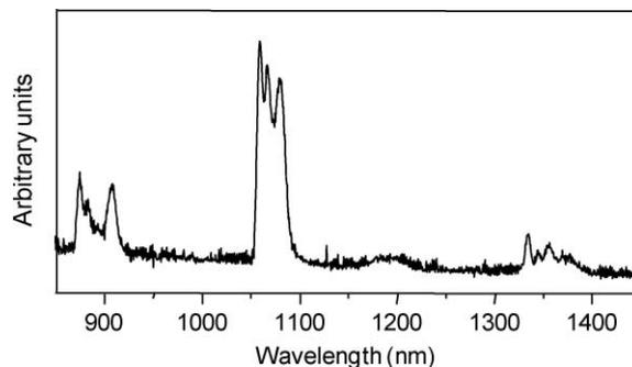
Fig. 9 Normalized NIR emission spectrum of a solid state sample of  $[\text{Nd}(\text{CTPD})_3]$  at 10 K ( $\lambda_{\text{ex}} = 400\text{ nm}$ ).
