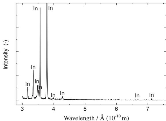
**Figure 2.** EPMA pattern of In-metal pellet obtained after milling  $\text{In}_2\text{O}_3$  and  $\text{Li}_3\text{N}$  mixture (molar ratio 1:3) for 120 min under  $\text{NH}_3$  gas environment.
