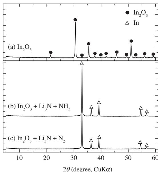
**Figure 1.** X-ray diffraction patterns of; (a) pure  $\text{In}_2\text{O}_3$  before milling, (b)  $\text{In}_2\text{O}_3/\text{Li}_3\text{N}$  mixture milled under  $\text{NH}_3$  gas environment; (c)  $\text{In}_2\text{O}_3/\text{Li}_3\text{N}$  mixture milled under  $\text{N}_2$  gas environment. All samples were milled for 120 min at 300 rpm.
