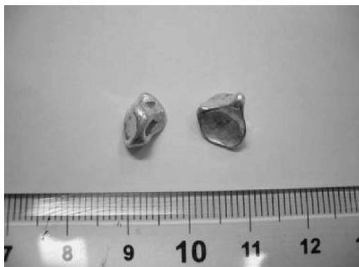
**Figure 3.** Photograph of In-metal pellet obtained after milling  $\text{In}_2\text{O}_3$  and  $\text{Li}_3\text{N}$  mixture (1:3 =  $\text{In}_2\text{O}_3$ : $\text{Li}_3\text{N}$  molar ratio) for 120 min under  $\text{NH}_3$  gas environment.
