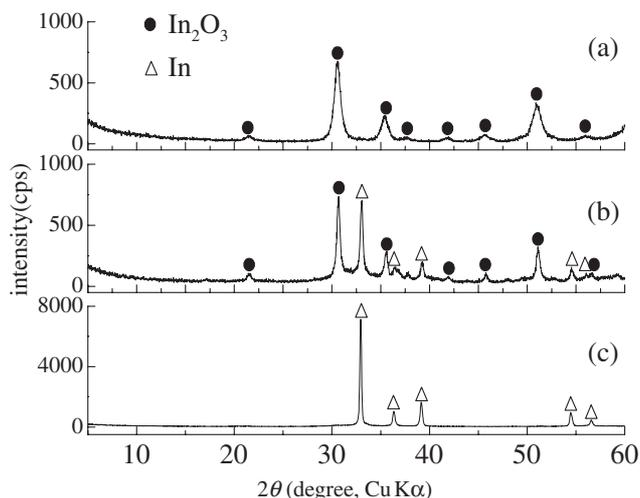
**Figure 4.** X-ray diffraction patterns of sample mixtures milled for 120 min at 300 rpm; (a)  $\text{In}_2\text{O}_3$  under  $\text{NH}_3$  gas; (b)  $\text{In}_2\text{O}_3$ / $\text{Li}_3\text{N}$  mixture without  $\text{NH}_3$ / $\text{N}_2$  gases; (c)  $\text{In}_2\text{O}_3$ / $\text{Li}_3\text{N}$  mixture under  $\text{NH}_3$  gas environment.
