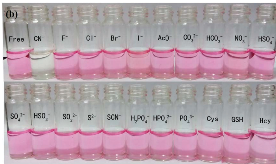
Fig. 4 (a) UV-Vis absorption spectra and (b) color changes of 1 in THF (10 \mu M) upon addition of 10 equiv. of each anion aqueous solution.
