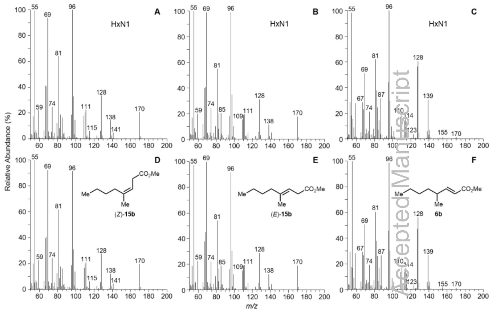
Figure 2. Mass spectra of compounds eluting at 21.42 (A), 22.07 (B) and 22.15 (C) min from methylated culture extracts of HxN1 (cf. Figure 1A) compared with the mass spectra of synthetic standards (Z)-15b (D), (E)-15b (E) and 6b (F).
