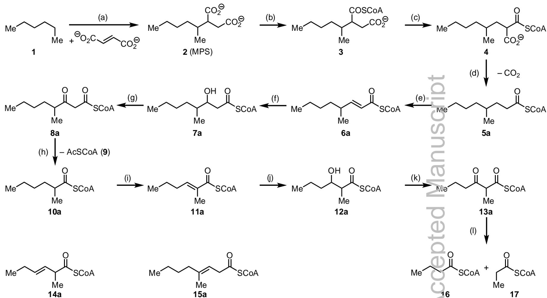
Scheme 1. Proposed pathway for the anaerobic degradation of *n*-hexane (**1**) by strain HxN1, for corresponding transformations (a) to (l) see text.
