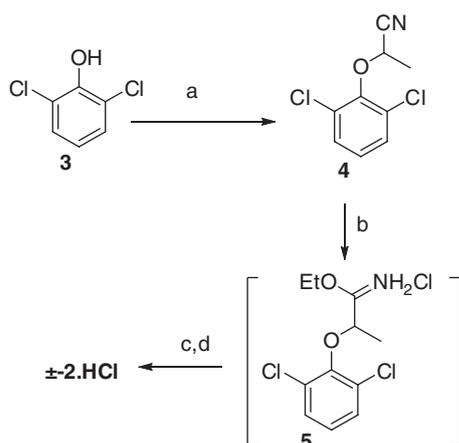
Reagents and Conditions: a.  $K_2CO_3$ , 2-butanone, 2-chloro propionitrile, reflux, 5h. b. HCl, ethanol, 0 °C, c. 1,1',2,2'- $d_4$ -ethylenediamine, EtOH, d. HCl,  $i$ -PrOH (68% over 2 steps)
