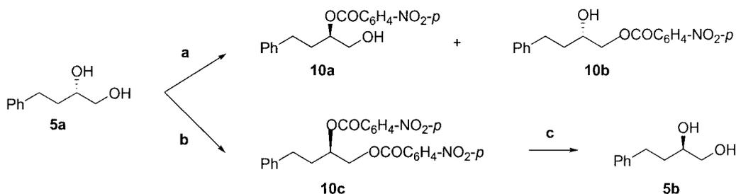
Scheme 2. Conditions and reagents: (a)  $\text{PPh}_3$  (1 equiv.), DIAD (1 equiv.),  $p\text{-NO}_2\text{C}_6\text{H}_4\text{COOH}$  (1 equiv.), THF, room temp., 2 h; (b)  $\text{PPh}_3$  (2 equiv.), DIAD (2 equiv.),  $p\text{-NO}_2\text{C}_6\text{H}_4\text{COOH}$  (2 equiv.), THF, room temp., 2 h; (c) catalytic Na, MeOH, room temp., 1 h.
