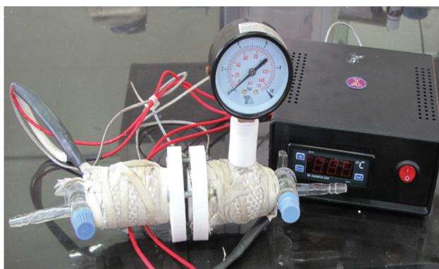
Fig. 1: Homemade catalytic membrane system cell.
