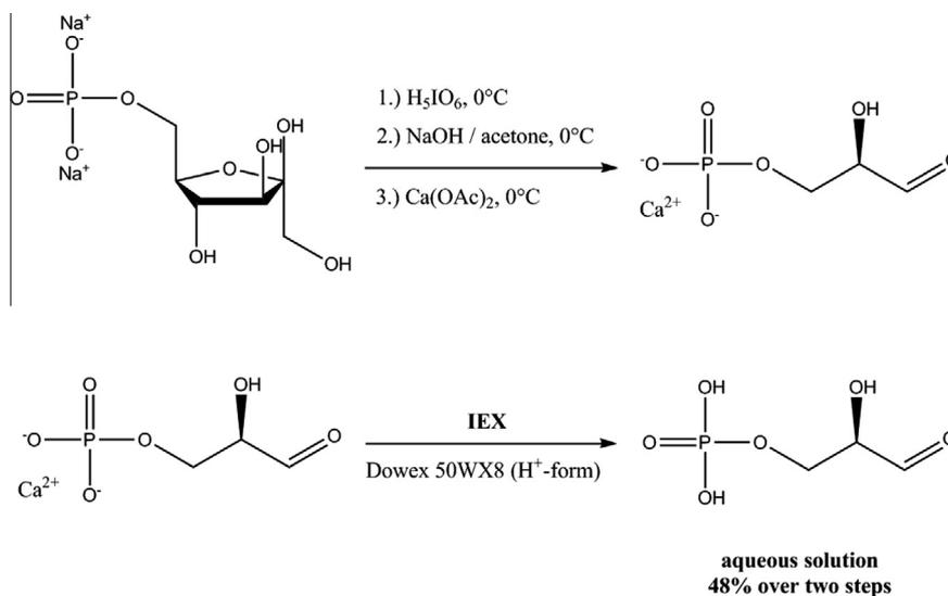
**Scheme 2.** Chemical synthesis of D-glyceraldehyde 3-phosphate. Step one is a modification of an already published method<sup>31</sup> to obtain the calcium salt of D-GAP. In a second step, the calcium salt was converted into the corresponding free acid of D-GAP by ion exchange.
