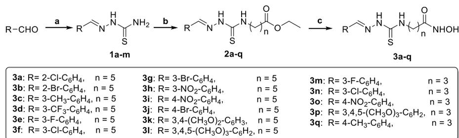
**Scheme 1.** Synthesis of compounds **3a-q**. Reagent and condition: a) Thiosemicarbazide, MeOH, 100 °C, 8 h; b) NaH, 1,4-Dioxane, Ethyl 6-bromohexanoate/Ethyl 4-bromobutyrate, reflux, 10 h; c) EtOH, NH<sub>2</sub>OH.HCl, KOH, -10 °C, 4 h.
