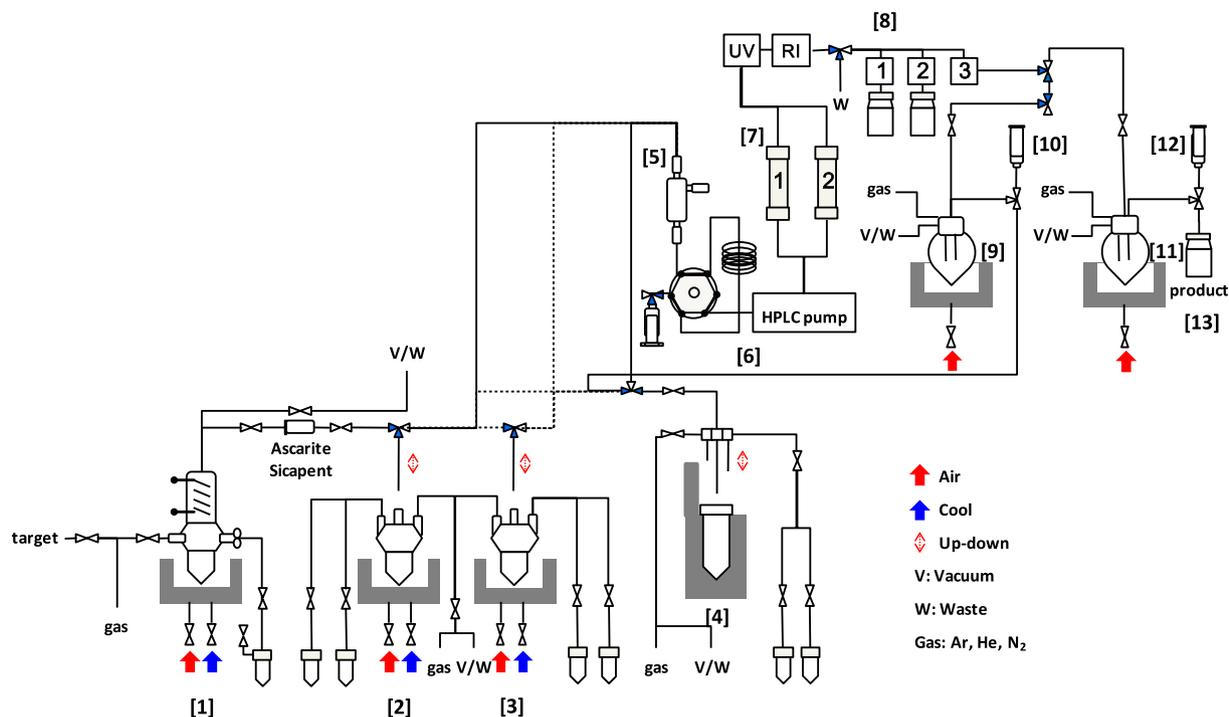
**Figure 4.** Automated radiolabeling system designed for sequential two-step-radiosynthesis of  $[^{11}\text{C}]\text{SC-62807}$ . [1] = reactor for  $[^{11}\text{C}]\text{CH}_3\text{I}$  production, [2] and [3] = reactor, [4] = microwave apparatus, [5] = reservoir, [6] = HPLC pump, [7] = column switching, [8] = fraction collector, [9] and [11] = evaporator, [10] and [12] = syringe, [13] = vial.
