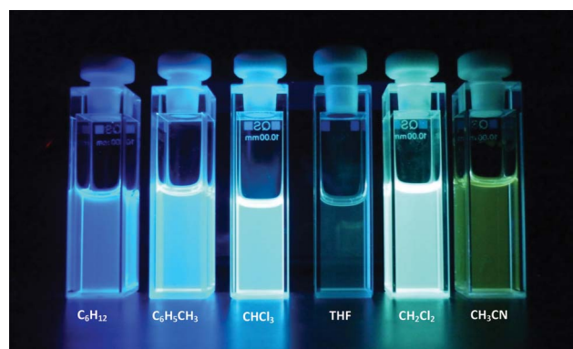
Fig. 3 Photograph of the emission of 7 in different solvents.
