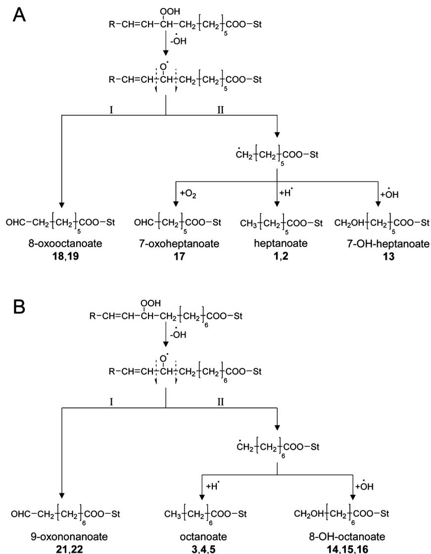
**Figure 6.** Formation pathways of steryl/stanyl ester oxidation products in the acyl chain by homolytic  $\beta$ -scission of primarily formed allylic hydroperoxides on positions (A) 8 and (B) 9. Adapted from Frankel.<sup>37</sup> Numbering corresponds to that in Figures 2 and 5. Only pathways leading to the compounds identified in this study are illustrated.
