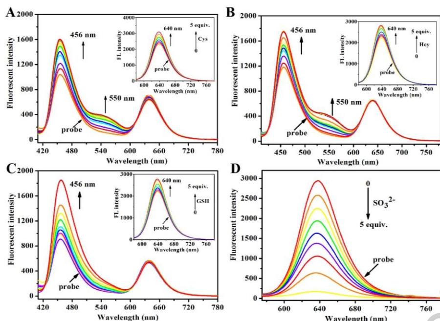
**Fig. 1.** Fluorescence spectra of PI-CO-NBD (10 μmol/L) with (A) Cys (0-50 μmol/L) (B) Hcy (0-50 μmol/L) (C) GSH (0-50 μmol/L) (D) SO<sub>3</sub><sup>2-</sup> (0-50 μmol/L) in the PBS buffer (pH 7.4, containing 20% CH<sub>3</sub>CN, v/v). λ<sub>ex</sub> = 395 nm, Ex/Em slit: 5/2 nm.
