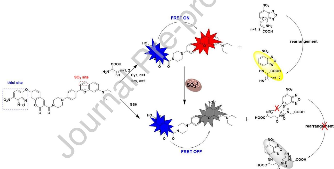
**Scheme 2.** Response mechanisms of PI-CO-NBD with Cys/Hcy/GSH and SO<sub>2</sub>.
