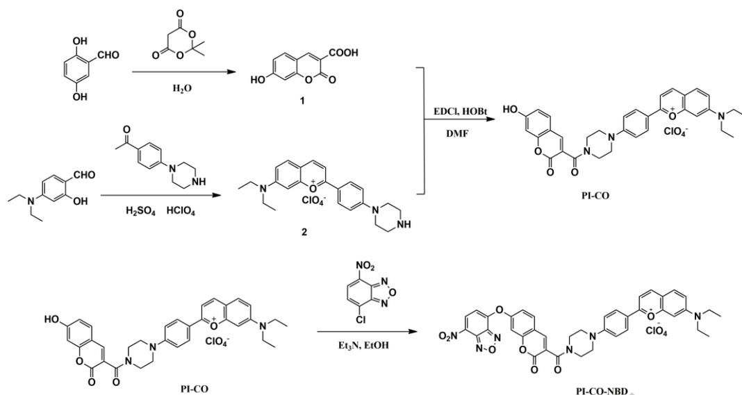
Scheme 1. The synthesis of the probe PI-CO-NBD.
