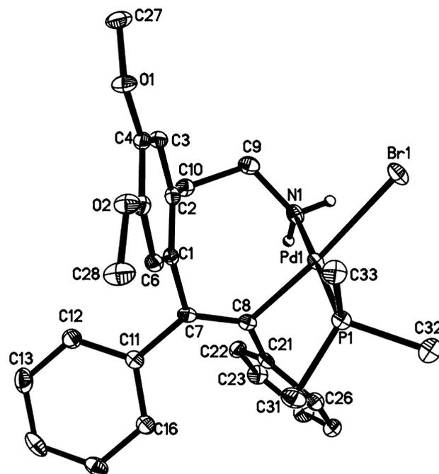
**Figure 2.** Thermal ellipsoid plot (50% probability) of complex **3a** along with the labeling scheme. The hydrogen atoms bonded to carbon have been omitted for the sake of clarity. Selected bond lengths (angstroms) and angles (degrees): Pd(1)–Br(1), 2.5237(3); Pd(1)–N(1), 2.1252(17); Pd(1)–C(8), 2.0091(18); Pd(1)–P(1), 2.2424(5); C(7)–C(8), 1.348(3); Br(1)–Pd(1)–N(1), 89.37(5); N(1)–Pd(1)–C(8), 87.01(7); C(8)–Pd(1)–P(1), 91.94(5); P(1)–Pd(1)–Br(1), 91.807(15).
