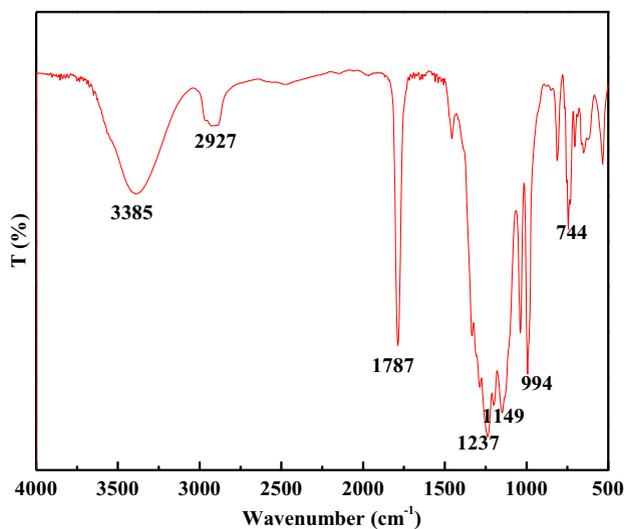
**Fig. 1** FTIR spectra of byproducts from glycidol and PFEF
