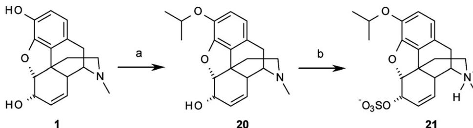
**Scheme 2.** Synthesis of 3-O-isopropylmorphine-6-O-sulfate (**21**). (a) 2-iodopropane, NaOEt, EtOH, reflux, 4 h. (b) Pyridine-SO<sub>3</sub>, pyridine, 60 °C, 3.5 h.
