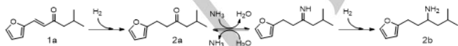
Scheme 2. Reaction pathway for the catalytic conversion of 1a into the furanic amine 2b over Ru/C.
