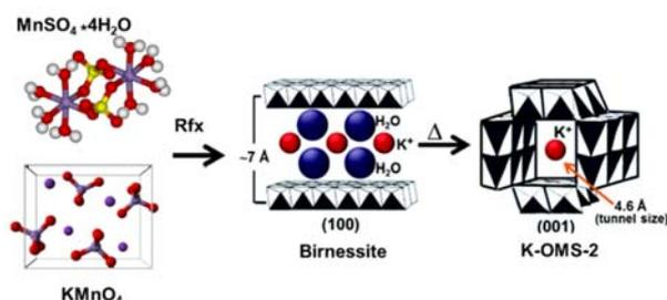
**Figure 2.** Schematic overview for the synthesis of K-OMS-2
