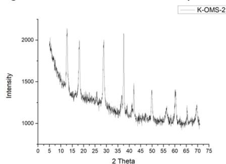
**Figure 3.** XRD-pattern of synthesized K-OMS-2
