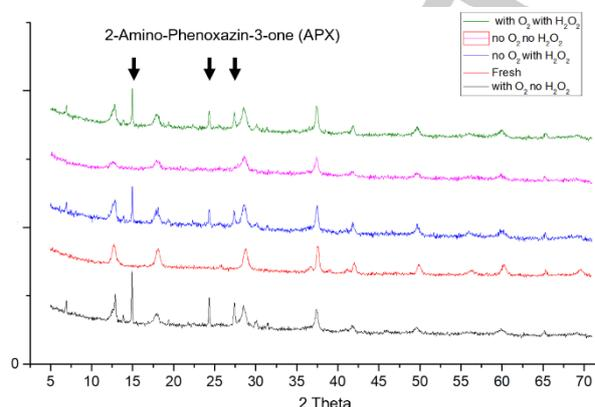
**Figure 4.** XRD-pattern of fresh and used catalysts
