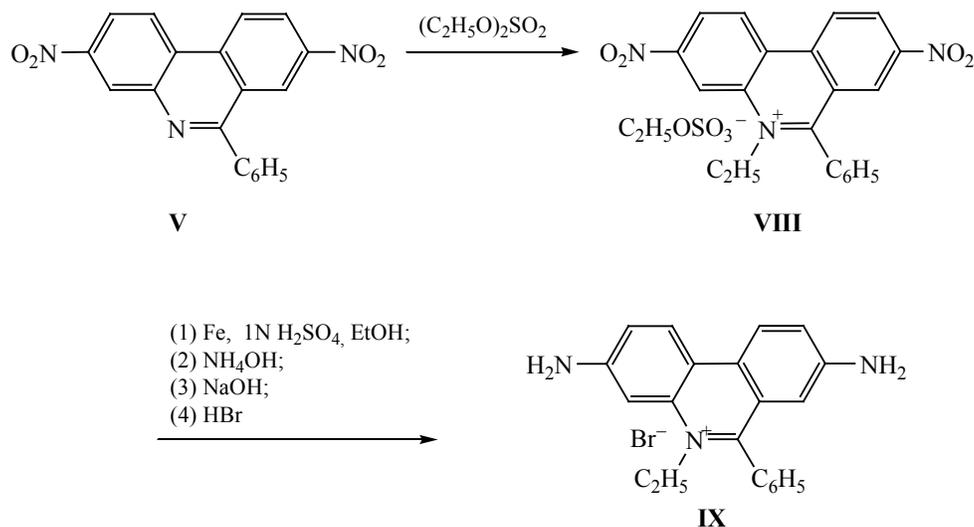
and 95% ethanol was used in the stage of reduction of ethyl sulfate **VIII** with powdered iron, which precluded formation of difficultly soluble products in hydrolysis of compound **VIII**.
